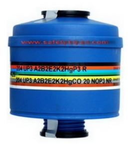
Combined filter with standard thread connector to **EN 148-1** for organic vapours having boiling point higher than 65 °C and inorganic gases and vapours, acid gases, Sulphur Dioxide (SO2), Ammonia (NH3) and its organic derivatives, Nitrous Oxides, Mercury Vapours, Carbon Monoxide (CO) and dusts, fumes, mists. The filter can be used with masks type **TR 82**, **TR 2002 CL2** and **TR 2002 CL3** or equivalent, provided that they are fitted with EN 148-1 connector.
